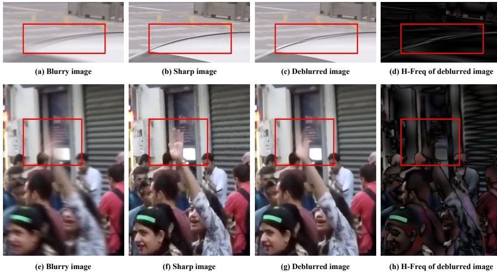
Fig. 1. The deblurring images of an existing representative DM, InDI [16]. The first row corresponds to the outlines of a car and second row corresponds to a human hand. The high-frequency component of the image is extracted using Fourier Transform. It can be observed that high-frequency components are likely to generate or exaggerate some unrealistic details and lead to local inconsistency due to the diffusion on irrelevant artifacts.
